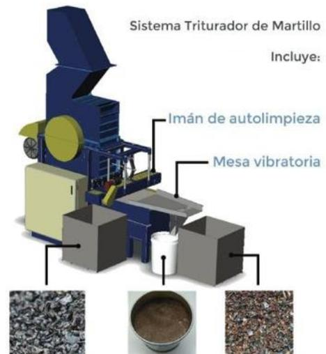
Ferrous Fraction Fines & Dust Non-Ferrous Fraction
